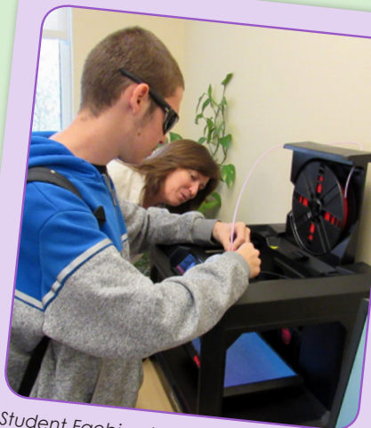
Student Faebian loads the raw materials (plastic filament strips) into a 3D printing machine as Librarian Ms. Amy Brody verbally guides him along the steps.
